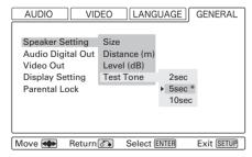
Select the Test Tone menu item, and choose between 2, 5\* and 10 seconds. This represents the length of time that the test tone is output from each speaker when Test Start is selected.
